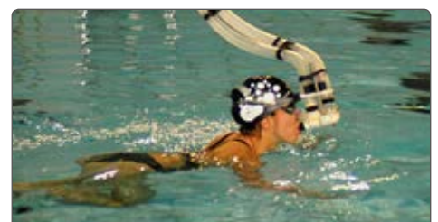
Possibility to measure gas exchange on swimmers in their environment (swimming pool or flume) with the optional snorkel Aquatrainer
